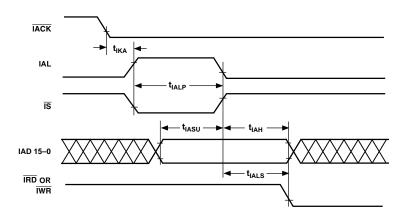
Figure 28. IDMA Address Latch
